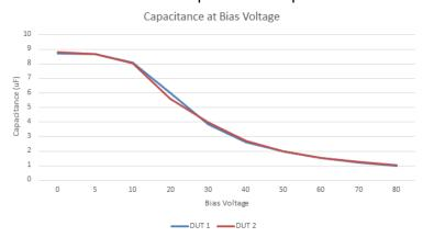
Graph above: Tested effective capacitance of the high voltage decoupling capacitors against applied bias voltage.
